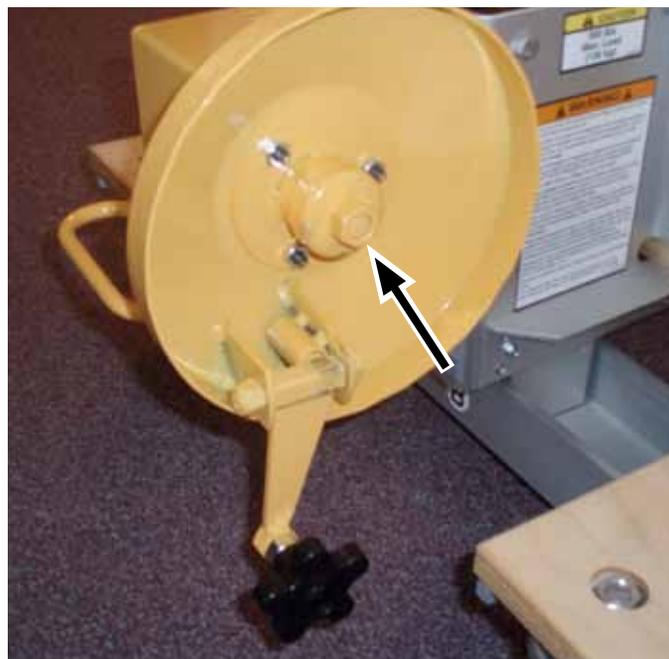
9) Install the Drill Drive™ winch hub (**NEVER** try to use a drill to operate your Drill Drive™ winch system without this hub securely installed).
