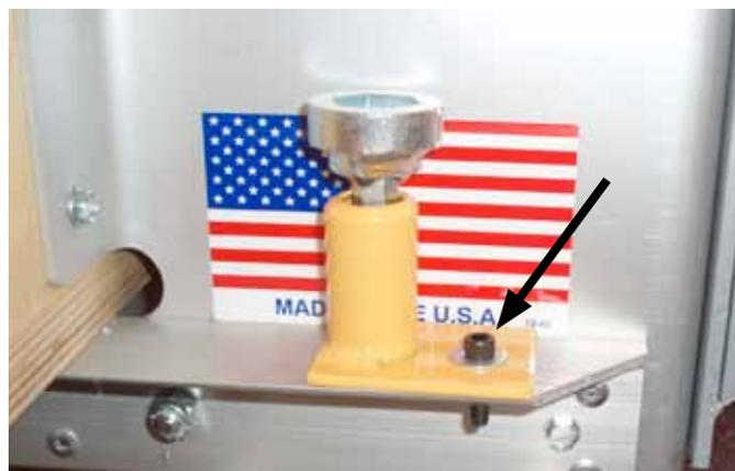
10) Install the storage post for the drill adapter.
