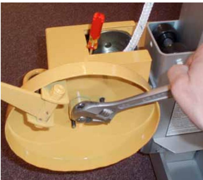
8) Install the winch nut and fasten securely in place. (You will find it helpful to lock the winch from rotating while tightening the winch nut by carefully inserting a small screw driver into the gear mechanism.)
