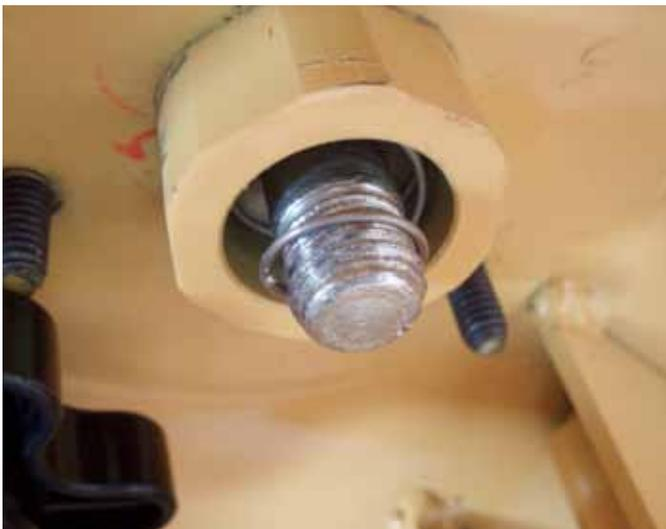
7) Install the winch handle spring as shown with the wide end in first and the narrow end out.
