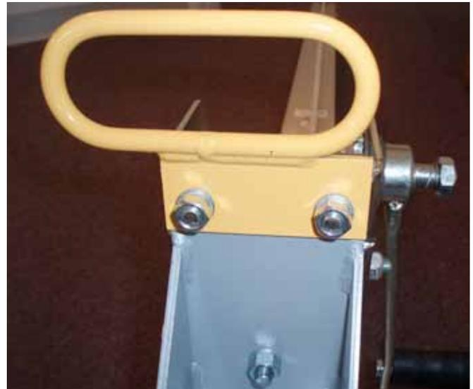
2) Install the grip handle as shown. Make sure the off set is to the left as shown to allow proper operation of the winch handle.
