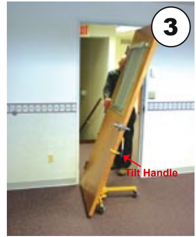
With the Tilt Handle down the Doorminator™ will roll through the door opening.
