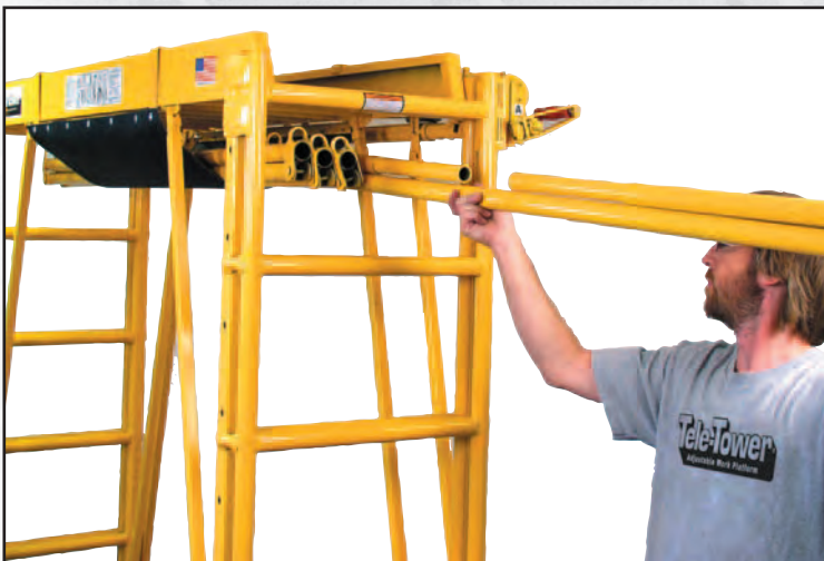
3. Install rails for on-board storage.
