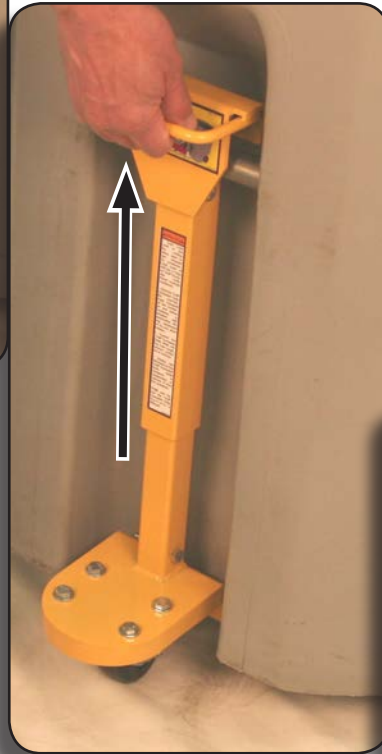
Hook the cross bar on the container
